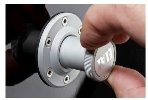
By means of an adjusting knob at the rear side of the speaker the whole VX-JET driver may be moved 8 mm out (in front of the baffle) or 8 mm in (behind the baffle). The idea behind is the fact that each room has its own acoustical behaviour and the same speaker produces different sounds in different rooms. The wish of "one speaker for all rooms" has been a myth ... until
